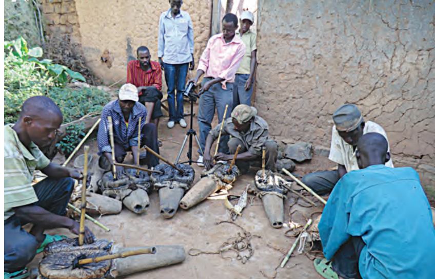
Experimental iron smelting in Central Rwanda, 2014. Before smelting starts, blacksmiths grease the sheepskins—the pot bellows covers—with cow butter to ensure suppleness. Damaged skin is replaced. These blacksmiths have reported that cow butter and smoke are the primary products used for conserving their bellows. Photo: Courtesy of the Rwanda Cultural Heritage Academy.
