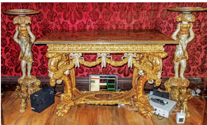
The Gole Suite in the Cartoon Gallery at Knole with acoustic emission monitoring equipment. Photo: ©National Trust/Nigel Blades.
