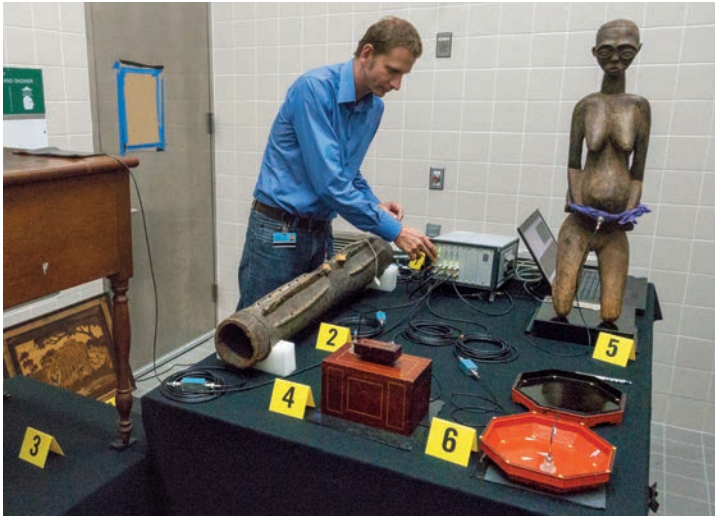
The MCE project's pilot study on climate-induced change to objects. Left: Michal Lukomski, senior scientist, assembles components for phase one of the study in the Getty Museum's conservation labs. The study included the use of acoustic emission to monitor the response of wood to climatic changes. Right: Joel Taylor, senior project specialist, discusses with Lukomski phase two of the pilot study, which was carried out on specially created mock-ups to better understand the extent to which different kinds of change could be measured. Photos: (left) Foekje Boersma, GCI, and (right) Andrzej Liguz, for the GCI.
