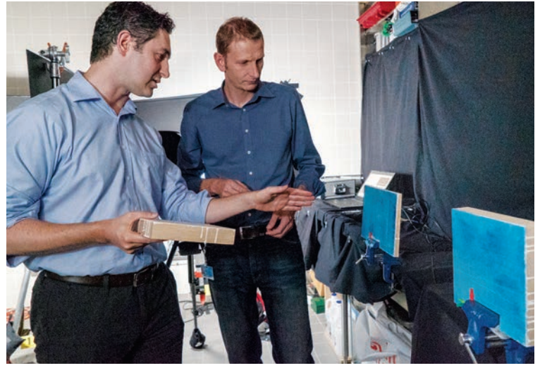
The MCE project's pilot study on climate-induced change to objects. Left: Michal Lukomski, senior scientist, assembles components for phase one of the study in the Getty Museum's conservation labs. The study included the use of acoustic emission to monitor the response of wood to climatic changes. Right: Joel Taylor, senior project specialist, discusses with Lukomski phase two of the pilot study, which was carried out on specially created mock-ups to better understand the extent to which different kinds of change could be measured. Photos: (left) Foekje Boersma, GCI, and (right) Andrzej Liguz, for the GCI.
