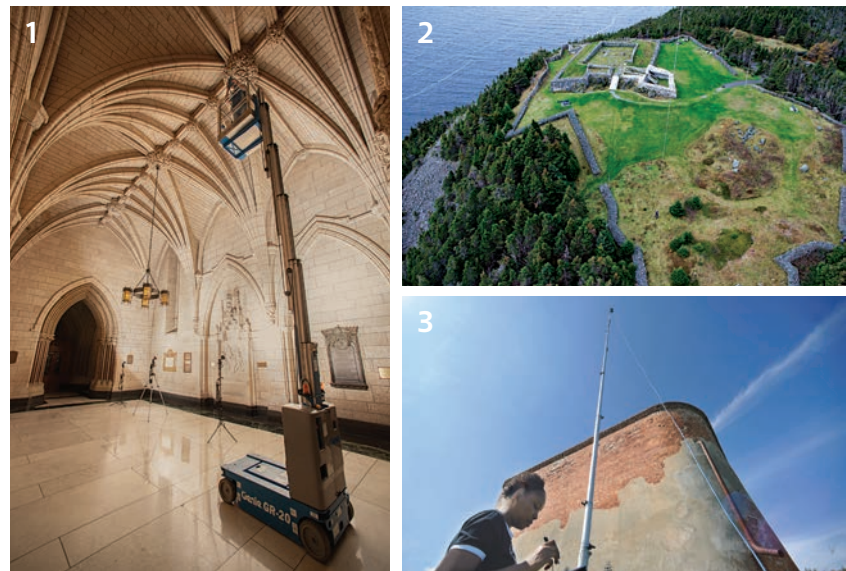
Various accessibility tools for photography used by Canada's Heritage Conservation Services (HCS), including (1) an elevated platform, (2) kite aerial photography, and (3) a photographic mast. Photos: HCS, Technical Services, Public Services and Procurement Canada.
