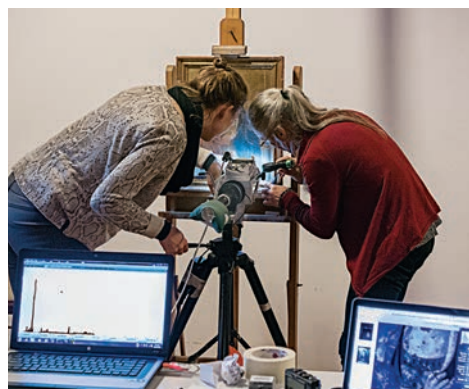
Participants in November 2016 Maastricht workshop engage in a hands-on exercise using a portable XRF unit. Photo: Stéphanie Auffret, GCI.
