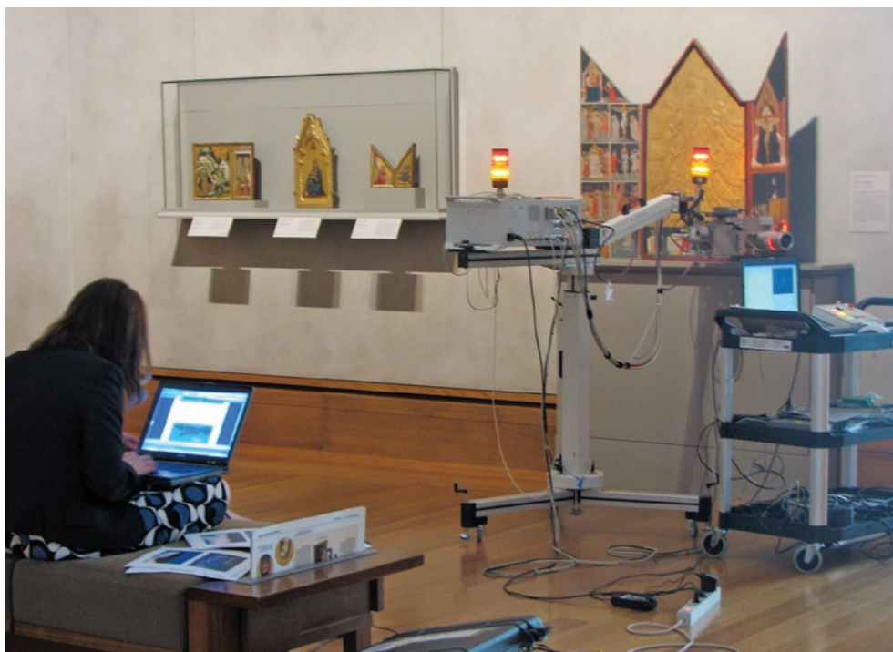
The ARTAX micro-XRF spectrometer acquiring element maps from figures in the Getty Museum's Chiarito Tabernacle . Photo: Karen Trentelman, GCI.
