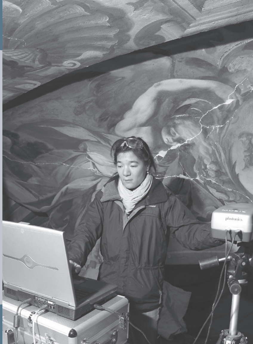
Lorinda Wong of the GCI using multispectral imaging to study the seventeenth-century wall paintings cycle by Andrea Pozzo at the Mission of Mondovi in Italy. Photo: Francesca Piqué.
