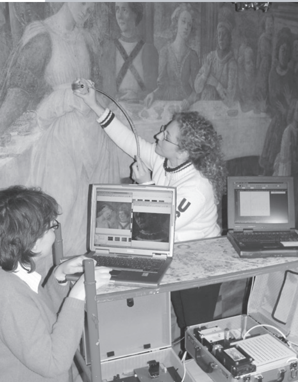
Catia Clementi and Ilaria Motta from the University of Perugia taking in situ measurements of the UV-visible fluorescence emission of organic materials in the Filippo Lippi wall paintings in Saint Stephen's Cathedral in Prato, Italy. Photo: Francesca Piqué.
