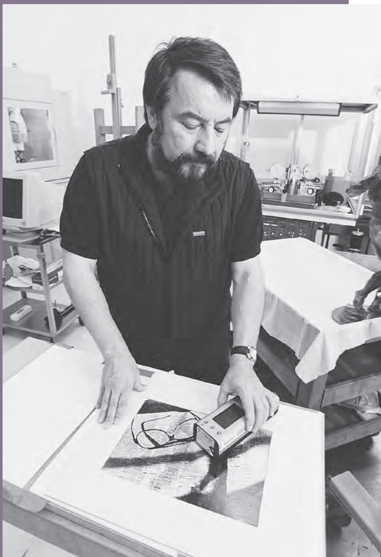
GCI senior scientist Dusan Stulik using a handheld XRF device to analyze the elemental composition of a photograph. Originally developed for the Mars Pathfinder project, the portable XRF is an example of the technological improvements advancing the analytical capabilities of conservation. Photo: Dennis Keeley.
