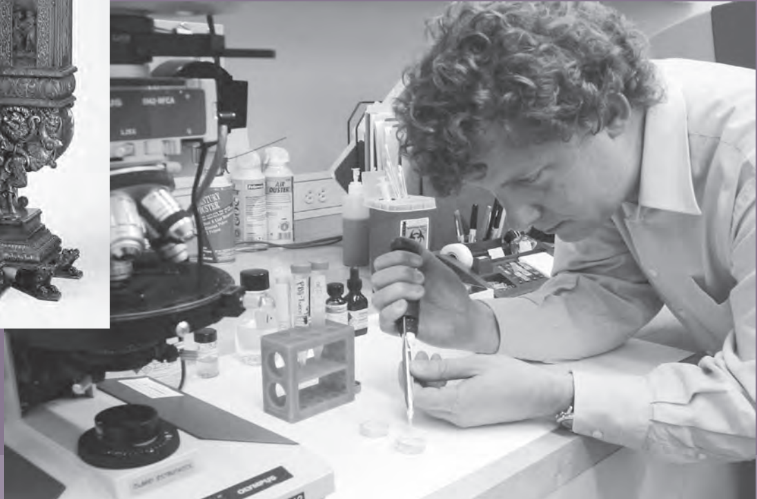
Below: Associate conservator Arlen Heginbotham of the Getty Museum applies fluorescent antibody stains to a cross section sample of paint from the cabinet. To precisely identify the materials and techniques used to create the cabinet's original surface, Heginbotham collaborated with staff from the USC Department of Biological Sciences. Photo: Brian Considine.
