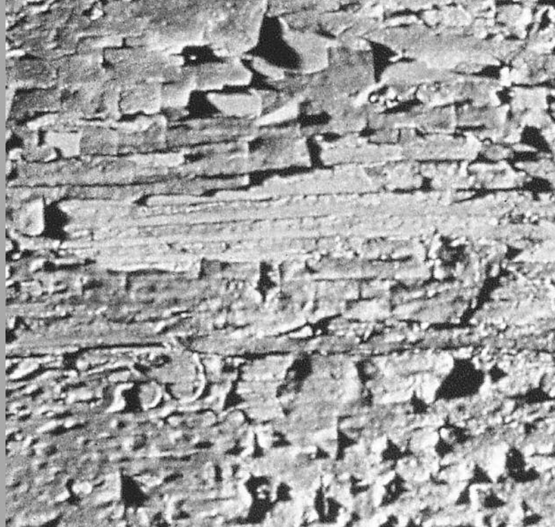
Details of two painted objects damaged as a consequence of environmental conditions. In the anonymous folk art painting on the left, the severely cracked surface is a result of widely fluctuating levels of relative humidity (RH). The flaking paint on the mid-19th-century wooden trade sign on the right was caused by low RH in a gallery that was heated but not humidified during the winter; all the flaking paint was readhered during conservation treatment in 1984, and the historic inn where the artifact is exhibited was climate controlled in 1993. Photos: Richard Kerschner; © Shelburne Museum, Shelburne, VT.
