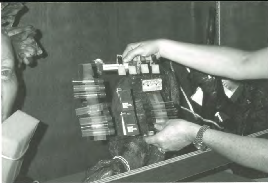
A set of passive monitors being placed in a display case at the Santa Barbara Museum of Art. The GCI has long been investigating ways to detect atmospheric pollutants that can threaten collections. Photo: Cecily Grzywacz.
