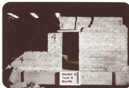
A one-fifth-size scale adobe model, unretrofitted, after being subjected to a series of simulated earthquakes.
