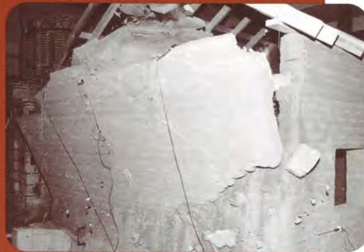
Left: The one-half-size scale model of a tapanco -style adobe with no retrofitting after the collapse of a gable end wall during testing on the shaking table in Skopje. Right: The gable end wall at the moment of collapse (the thin cables visible on the wall were part of the testing's instrumentation and not retrofitting).
