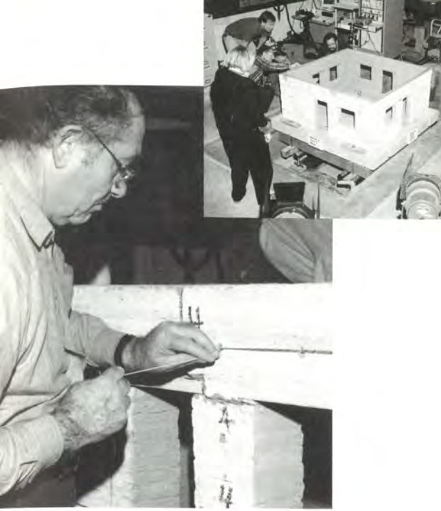
Top: Members of the Getty Seismic Adobe Project team examine an adobe model after it has been subjected to a simulated earthquake. Bottom: Bill Ginell, the GCI's director of the project, adjusts nylon straps on the model, designed to reduce shifting of adobe blocks during a quake. Photos: Louise Walker.
