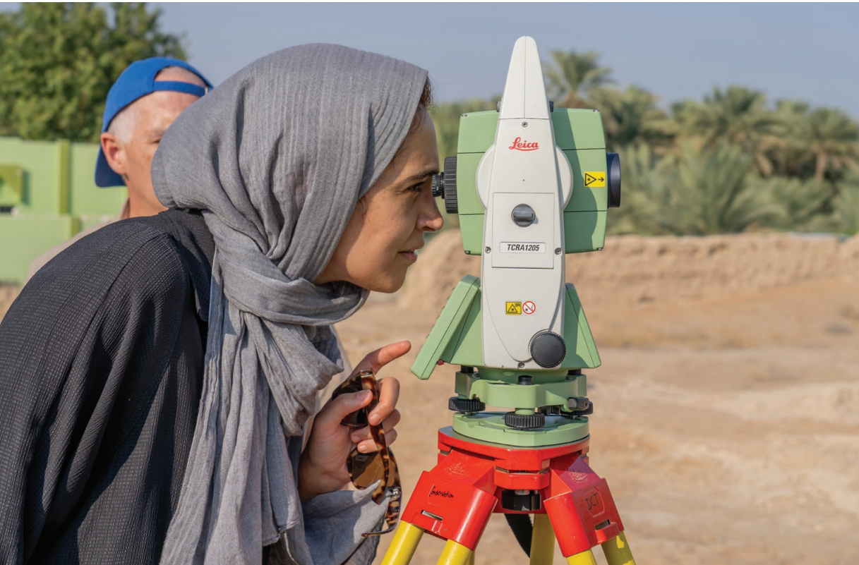
Zahra Ali Baba looks into a Total Station surveying instrument. Image courtesy of the Department of Culture and Tourism – Abu Dhabi
